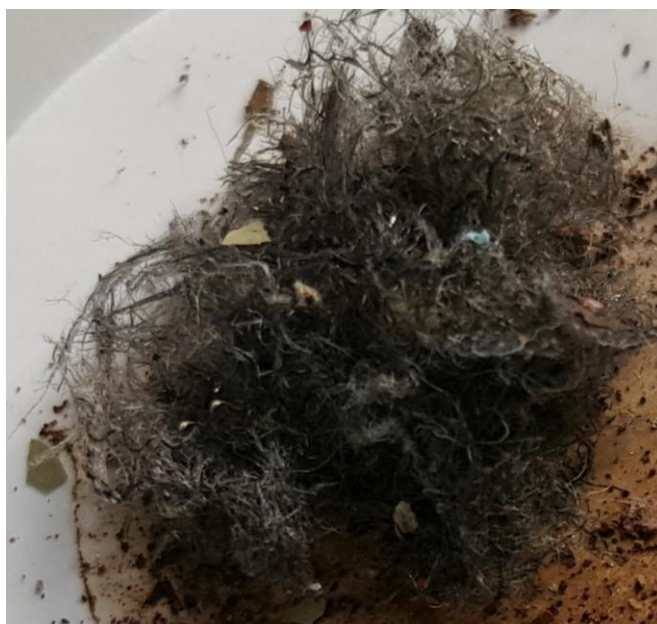
Figure 1.1 Filter membrane with fibres, sample 12345.001 – Fibres from Lube Oil Filters
