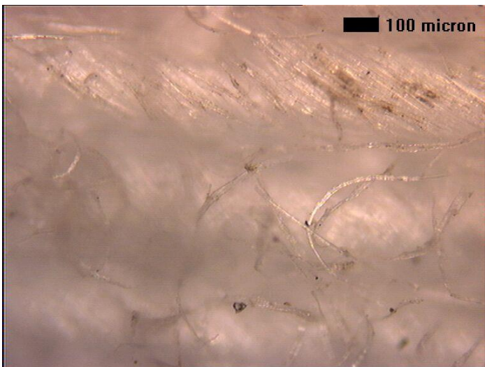
Figure 1.3 Microscopic view of Rag and Absorbent Pad fibres, samples 12345.002 and 12345.003
