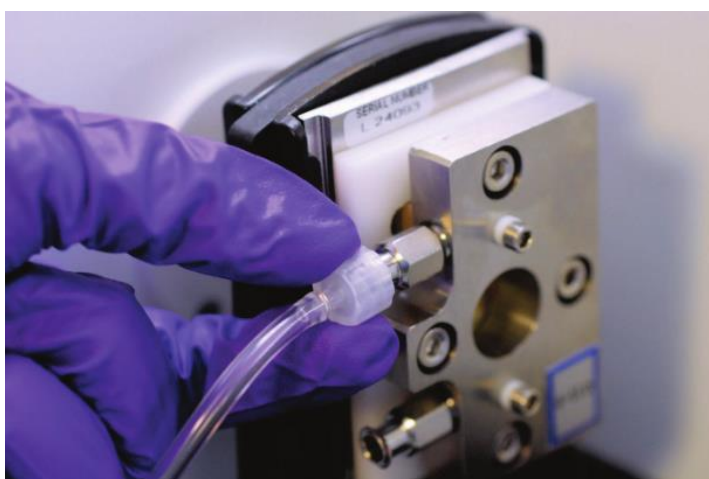
Figure 2.1 FTIR Transmission Cell and Perkin Elmer Spectrum Two FTIR Spectrometer with a Diamond UATR Accessory fitted
